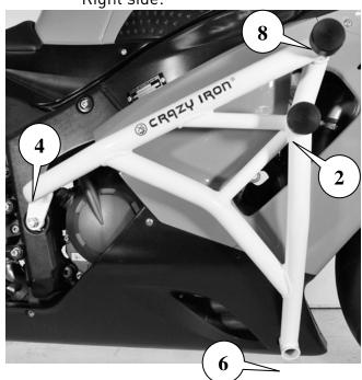
Bolt M10x1.25x70 - 1 pc. Bolt M10x1.25x40 - 1 pc. Washer - 2 pc. Spring washer - 2 pc. Plate (look at pic.) - 1 pc. spacer 20x10x10 - 1 pc. slider - 1 pc. bolt M6x16 - 1 pc. Screw the plate (look at the pic on the right) with bolt M10x1,25x70 through spacer 22x10x10 to the frame of motorcycle at the point 1. Then screw cage with bolt M10x1,25x40 to the plate.
